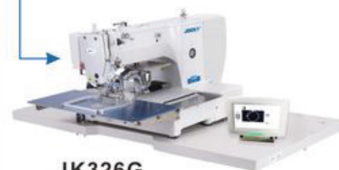
JK326G Pattern sewing machine with CH device
